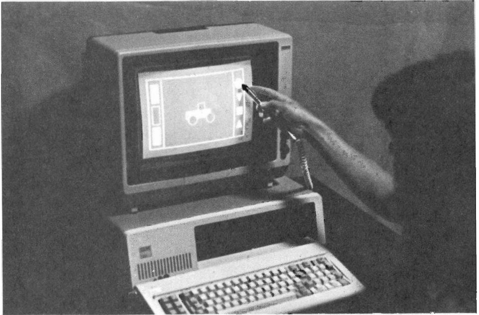
Figure 6-4 Light pen being used to make a menu selection.
